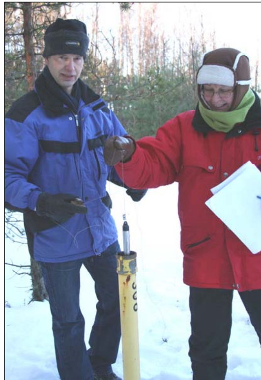
Figure VI—4 Groundwater monitoring tool installation at the well HP0306. (Photo by S. Luoma)
