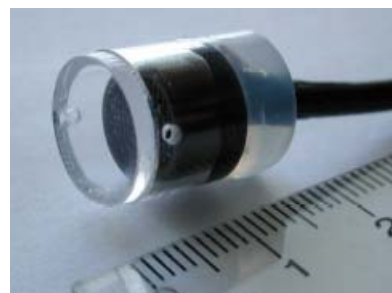
Figure 13 Q-BREATH sensor from Høk Instruments AB
