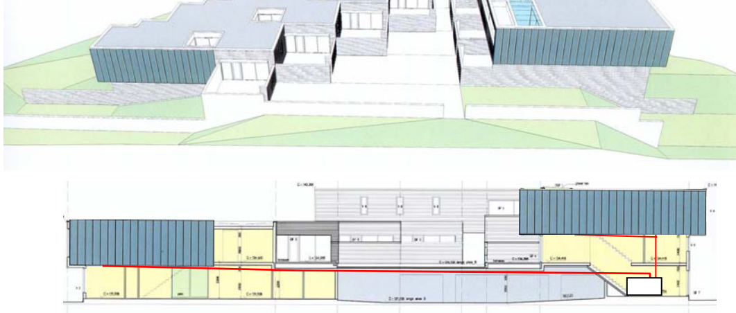
Fig.14 Schematic drawing of the multi-apartment complex at Bjørnveien 119 in Oslo (top) and solar collector system with piping and heat store in the technical room (bottom); Source: DDB arkitekter, Oslo, Backe Gruppen AS.
