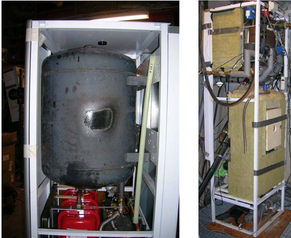
Fig. 10. Left: Top of the technical unit with a standard 80 liter auxiliary tank instead of a gas boiler. Right: Prototype of a technical unit at SERC with a cubic 80 liter tank in the top and an adapted pellet stove below.
