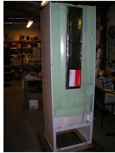
Fig.2 Left: View on the top of the tank with vacuum panels at the sides and the 2 small holes for the temperature sensors in the middle of the tank; Right: View at the front of the tank without the cover plate to see one of the vacuum panels.
