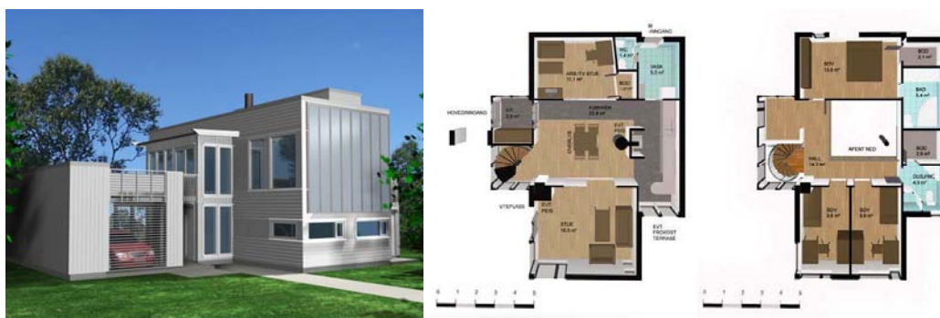
Fig.12. Type-house KARAKTER, example of a standardized single-family house for mass production with façade collectors (left); plan of the 1st floor (middle) and of the 2nd floor (right) (Source: Systemhus).
