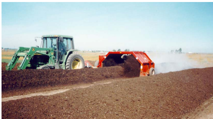
Figure 1 Typical Windrow Composting System
