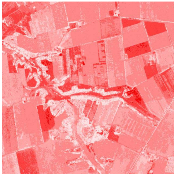
Figure 5.5. Signal strength –the difference between the initial signal and the reflected one. The denser the canopy, the weaker the reflected signal will be. The brighter the colours are the denser canopies.
