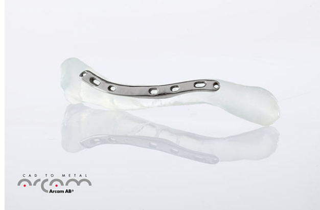
Figure 8.4 Individual boneplate made in Arcam EBM process
