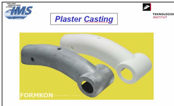
Figure 7.5 Plaster cast parts made of aluminium (Formkon)
