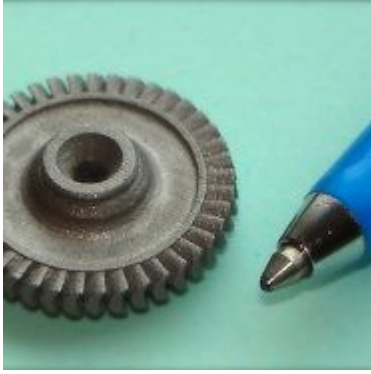
Figure 8.3 Small turbine wheel in stainless steel
