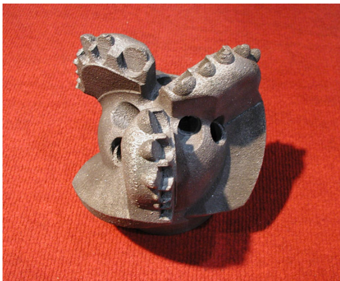
Photo 6.3 Drill-bit and impeller, made using the Arcam EBM process.
