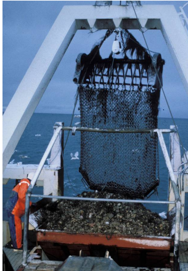
Figure 1.9 Roller scallop dredge used in Iceland.
