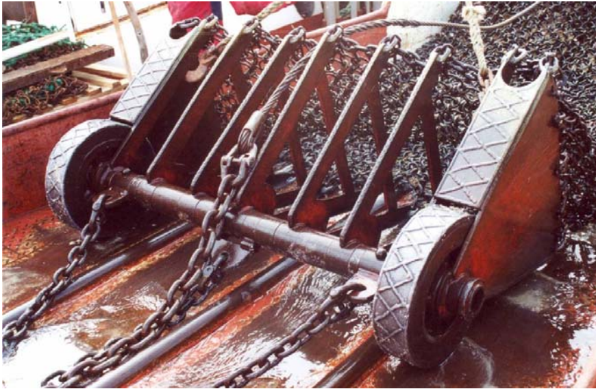
Figure 2.7 The roller dredge used in Iceland. The stone guards can spin around the axis, allowing the dredge to slide over boulders.
