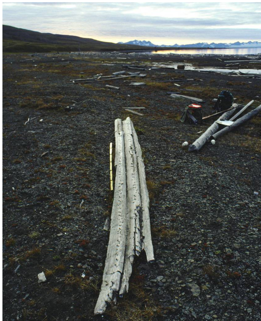
Figure 5.17 Part of a wrecked Pomor lodja, at Coles Bay in the Isfjorden, Spitsbergen. The lodjas were sewn vessels, varied in size, but capable of carrying gear, provisions and men for winter hunting expeditions to Svalbard. Lodja parts and wreckage are found all around the shores of Spitsbergen.
