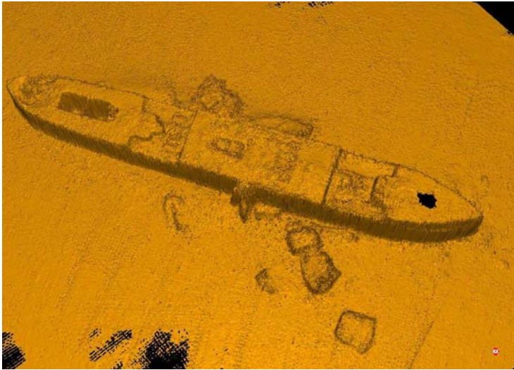
Figure 5.46 Wreck of a merchant ship in the harbour of Narvik recently recorded by the Norwegian Government Seabed Mapping Agency (Statens Kartverk, Sjøkartverket (SKSK)). The sonargram has high detail resolution; still higher resolution is available, depending on the hardware used, and software processing programs. This picture was recorded with a EM300 echo sounder, and modelled on a 0,25m grid. (Illustration by SKSK, http://www.mareano.no/ ).
