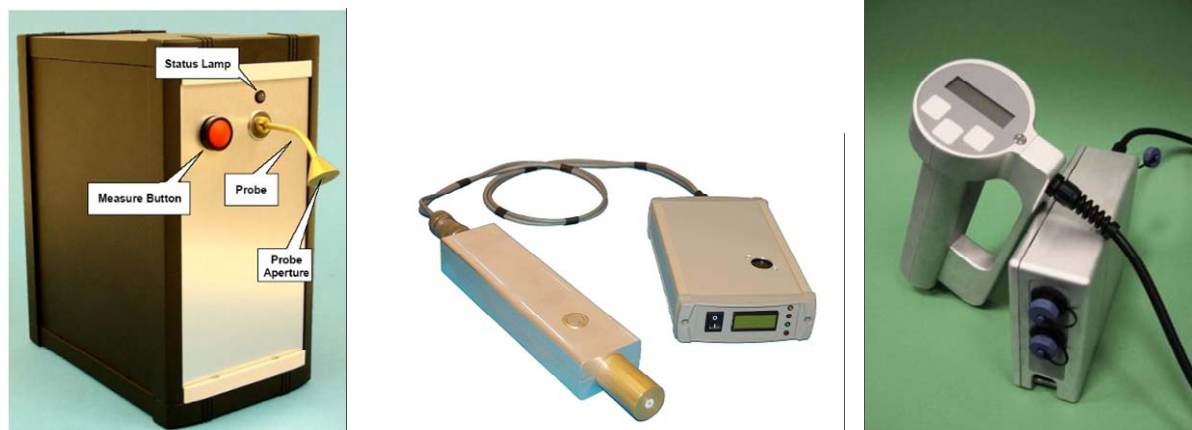
Figure 2 Three versions of MW-measurement equipment used in the project; from left to right; (i) the TDR – Instrument, Prototype TDR 1st Generation, CAU Kiel (P1), (ii) the TDR Sensor, Prototype hand 3rd Generation SEQUID GmbH (P3) and (iii) the RFQ Scan 3.0, hand held, SEQUID GmbH (TDR- Time domain reflection)
