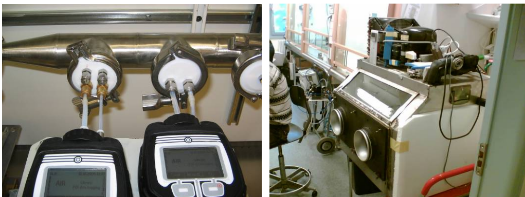
Fig.18. Two ChemPro units mounted on the agent generation test system and a climate control chamber for cold and hot temperature tests.
