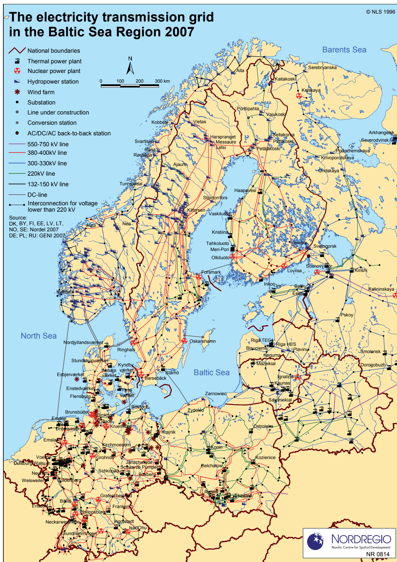
Figure 46: Energy transmission grid in the BSR
