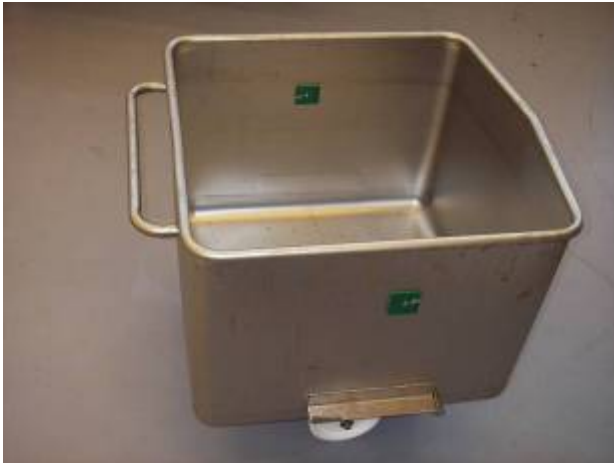
Figure 28. The RFSAW tags outside and inside an empty trolley.
