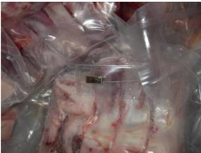
Figure 29. RFSAW-tag embedded among the meat products.
