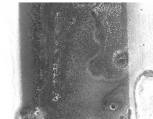
Fig. 4.1.6. a) The element thickness of ER probes pH 9.35 (in 25 mM K 2 HPO 4 or 22 mM NaOH) is under 50 ppm hydrogen sulphide atmosphere in an 11 day experiment with b) photo of the electrode exposed to 22 mM NaOH (50x).
