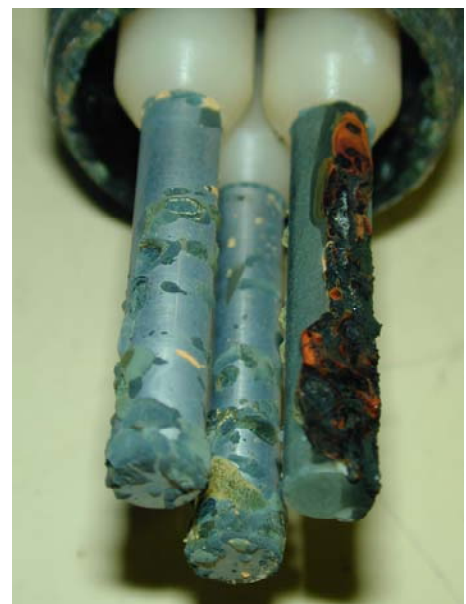
Fig. 4.3.51. Probes after a period of increased oxygen in Oskjuhlid station.
