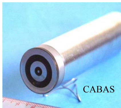
Fig. 3.3.2. Two types of localized corrosion probes applied for MIC. CABAS cell consist of concentric electrodes with the small anode in the center.
