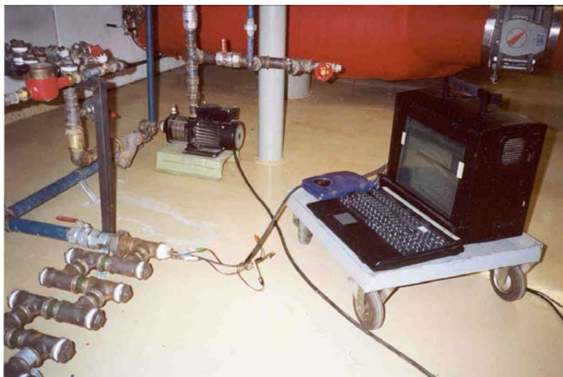
Fig.. 4.3.43. Corrosion test unit set-up at Oskjuhlid.
