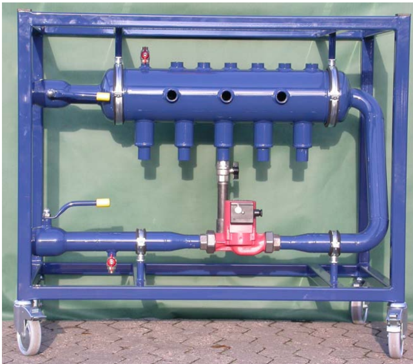
Fig. 4.6.10. Redesigned bypass unit shown without probes.
