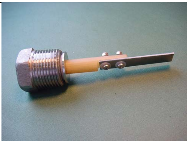
Fig. 4.2.25. Weight loss coupon. (Force Technology).
