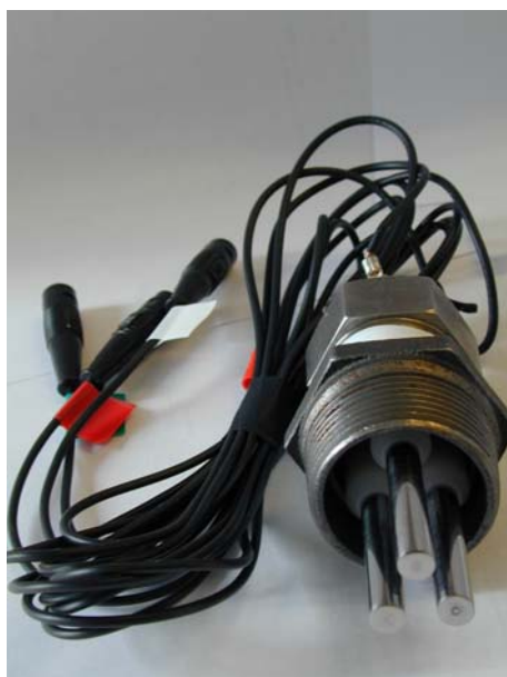
Fig. 4.3.44. Three electrode probe constructed at DTU.
