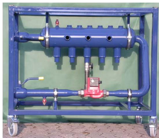
Figure 1b. Photo of bypass-unit with circulation pump before probe mountings.
