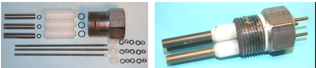
Fig 4.3.12. Three electrode probe type used in Ballerup and all other field units.
