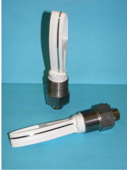
Fig. 4.2.3. DHS ER-probe design.
