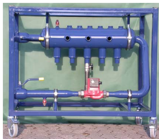
Figure 1b. Photo of the bypass-unit with circulation pump before probe mountings.
