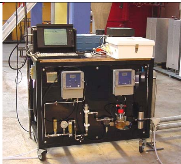
Fig. 4.2.24. Panel mounted on side stream unit during operation.
