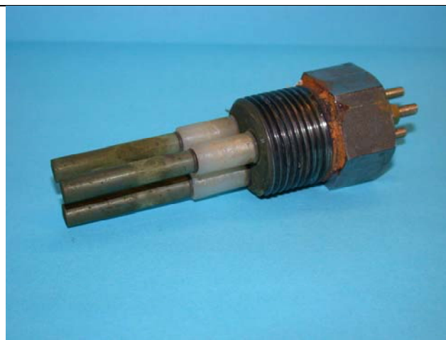
Fig. 4.2.26. Three-electrode probe for electrochemical measurements. (Technical University of Denmark).
