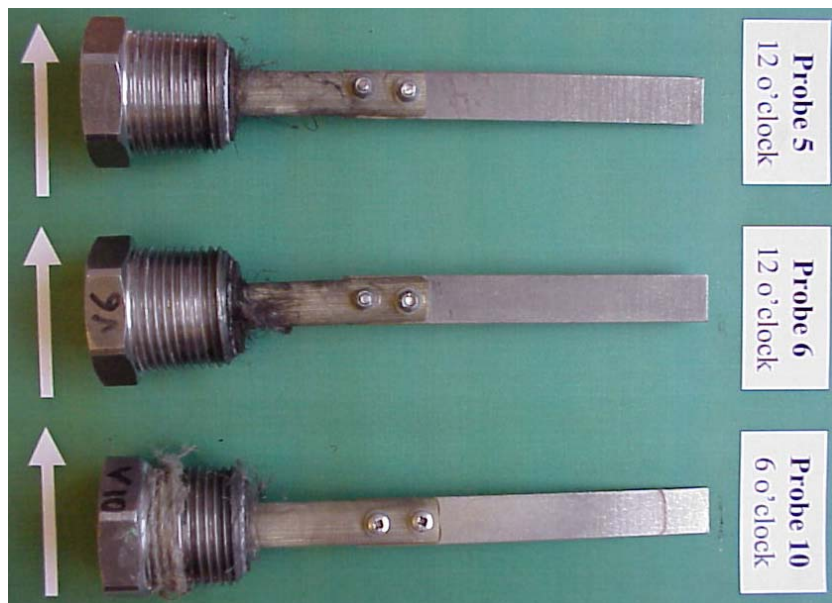
Photo 2. Overview of weight loss coupons probe 5 - 12 o'clock, probe 6 - 12 o'clock and probe 10 - 6 o'clock.
