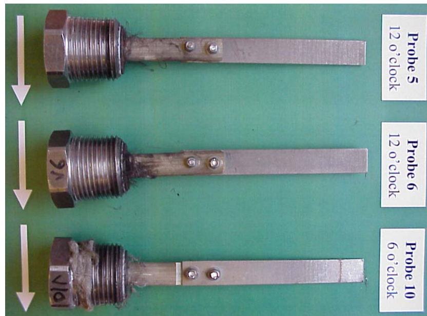
Photo 1. Overview of weight loss coupons probe 5 - 12 o'clock, probe 6 - 12 o'clock and probe 10 - 6 o'clock.
