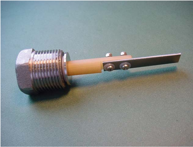
Fig. 4.6.11. New design of weight loss coupons with carbon steel disc for bio analysis.
