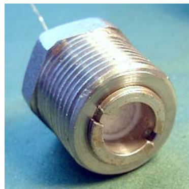
Fig. 3.3.4. Left: The LOCOR-CELL ® shown schematically as mounted in a steel pipe. The corrosion current is measured between the steel pipe surface and the pure steel anode using a zero resistant ammeter. Right: Photo of the LOCOR-Cell ® .
