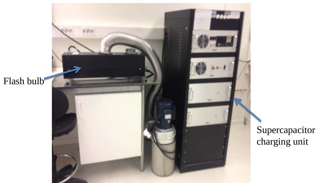
Figure 8. Flash sintering system capable of producing up to 2000W of UV-VIS light in 1 millisecond on a 30 cm x 2 cm area. The combination of high energy input on a short time scale allows for extremely fast temperature up- and down ramping which makes it possible to sinter metals and ceramics on temperature sensitive substrates such as cellulose based paper and plastic without significantly damaging the substrate
