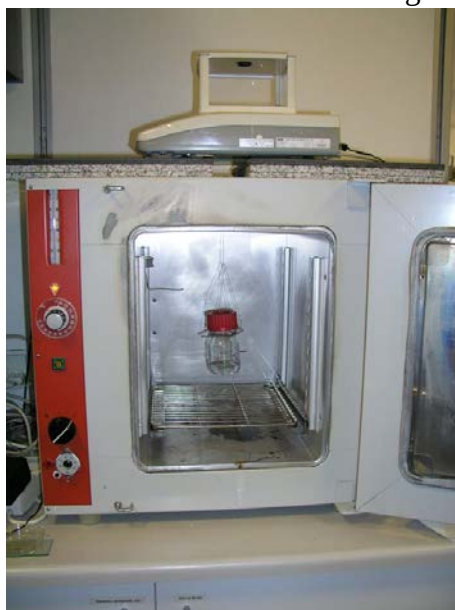
Figure 8: Setup using continuous weighing of suspended container
