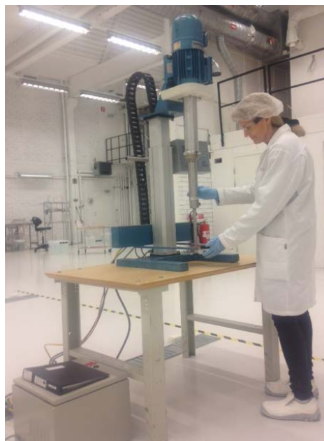
Figure 7. Dispersing and bead milling equipment capable of producing ink volumes up to 20 liters per batch.
