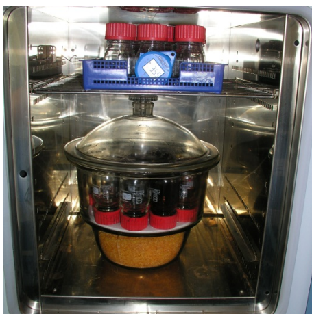
Figure 7: Parallel test with water vapour and liquid electrolyte
