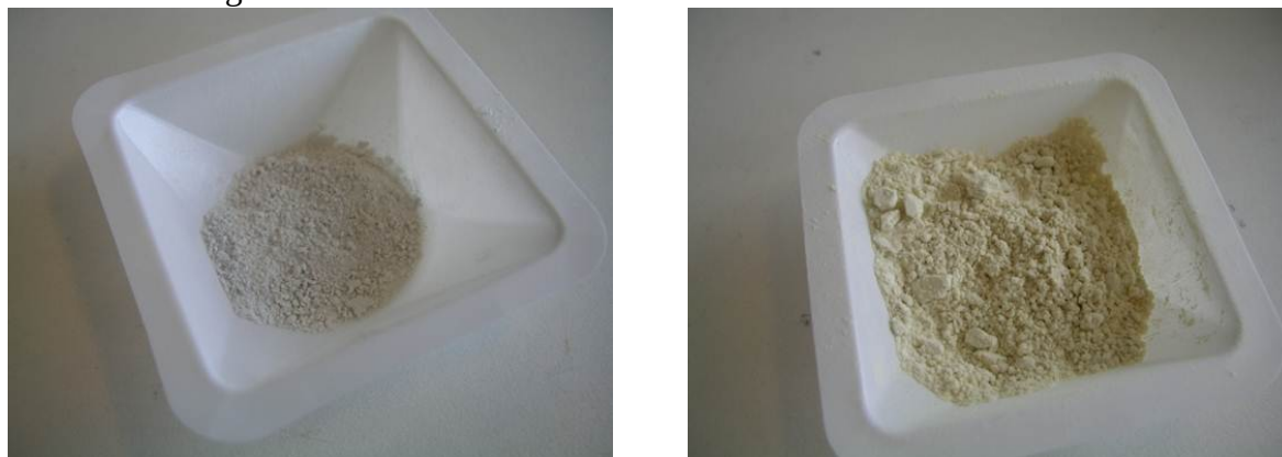
Figure 13: Left: Fine PCTFE particles ready for sealant use. Right: Fine LCP particles ready for sealant use
