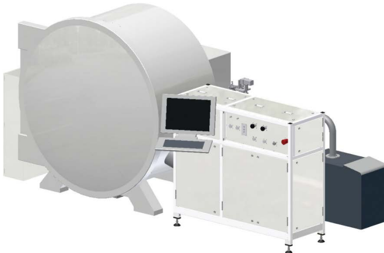
Figure 9: A schematics of Beneq's first roll to roll ALD coater for flexible films
