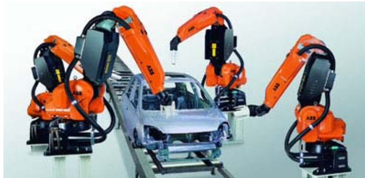
Figure 9.26 Paint robots from ABB AS, Robotics. The FlexLine system is a fully integrated paint system combining all advantages of cutting edge technologies.
