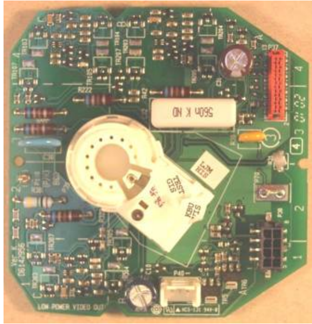
Figure 9.2 Low Power Video Output (LPVO) printed circuit board. Key parameters: 221 components total, 73 different components, 12 component suppliers, FR4: 2 layer, 1.6 mm thickness.
