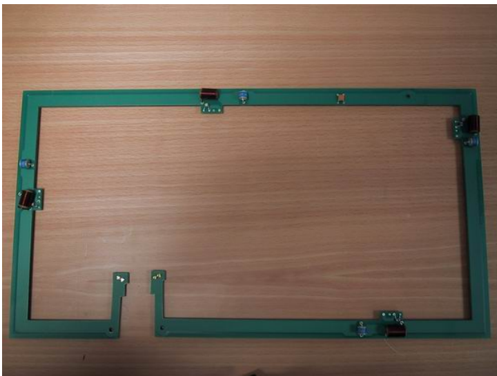
Figure 9.45 Antenna for Balise shown in Figure 9.46
