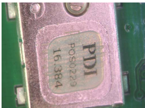
Figure 9.20 Components IDU unit. Greased label (left), Tantalum Capacitor slightly discolored (right)
