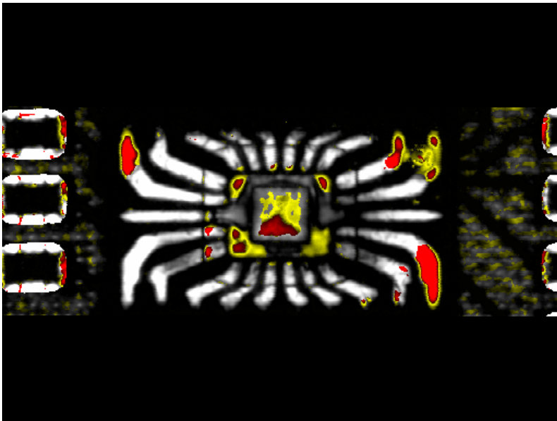
Figure 9.29 SAM image of a SO-20 package showing indications (red areas) of delamination in the leadframe/encapsulant interface areas with possible openings from the outside environment into the stitch bond areas. In addition, there are indications of delaminations in the die pad/encapsulant interface areas.
