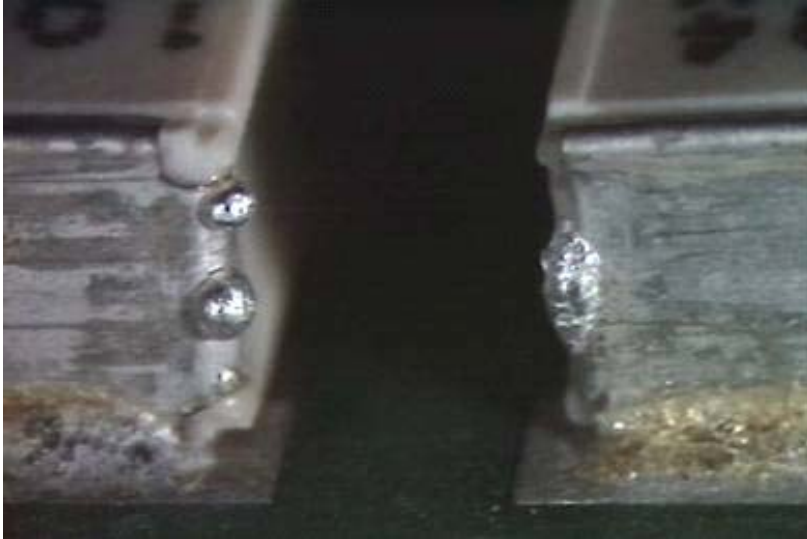
Figure 9.4 Tin-lead soldered internal interconnects become critical! Example: Polypropylene foil capacitor. Soldering condition out of specification, Peak temperature specified: Max. 220 °C, Time above 180°C: Max. 60 s, Lead free condition: 235 °C, 60 s
