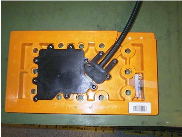
Figure 9.46 Balise before final assembly. Antenna is cast into the outer part of the structure.
