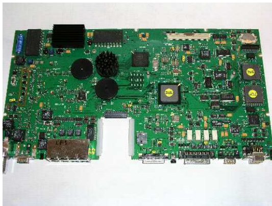
Figure 9.14 IDU-board. FR4-board, 410 mm x 220 mm x 2.4 mm, NiAu surface
