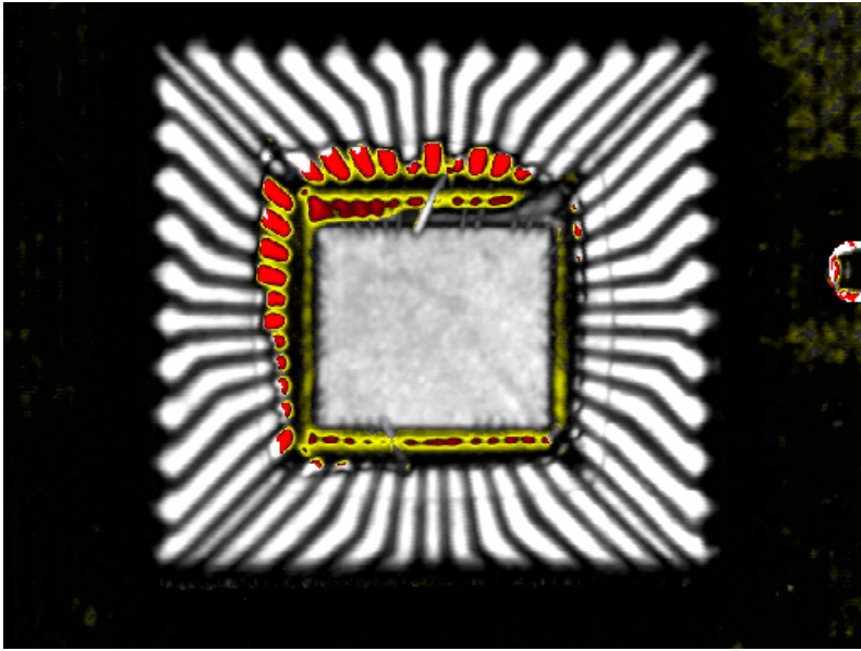
Figure 9.28 SAM image of QFP package showing indications (red areas) of delamination in the leadframe/encapsulant interface and in die pad/encapsulant interface areas.
