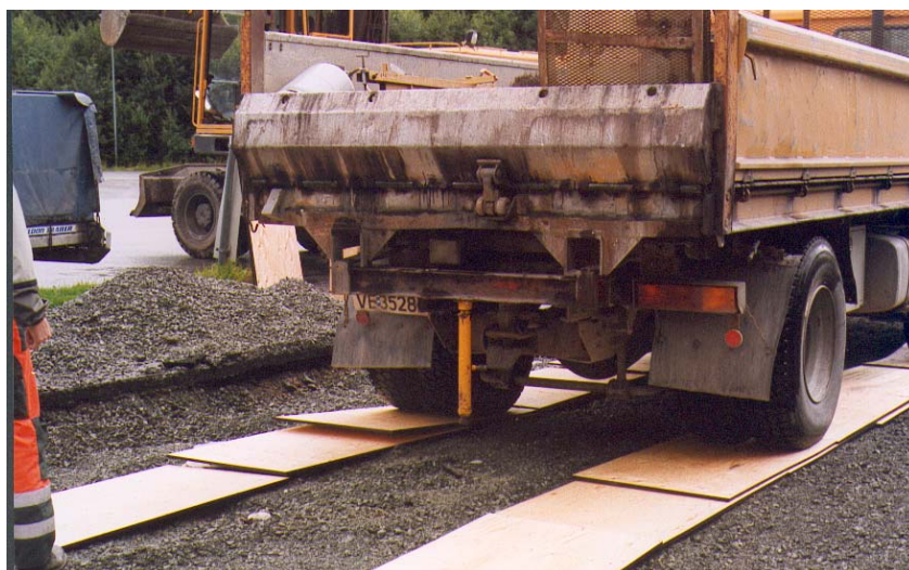
Figure 4.12 Plate loading test directly on LWA layer.
