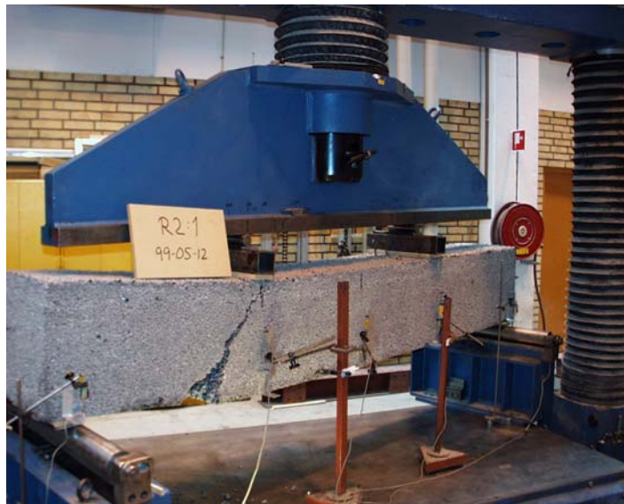
Figure 4.5 Full scale testing of LLP
