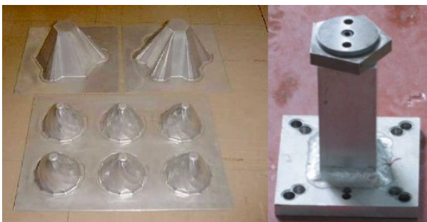
Figure 15 Simple support tool and parts made with it
