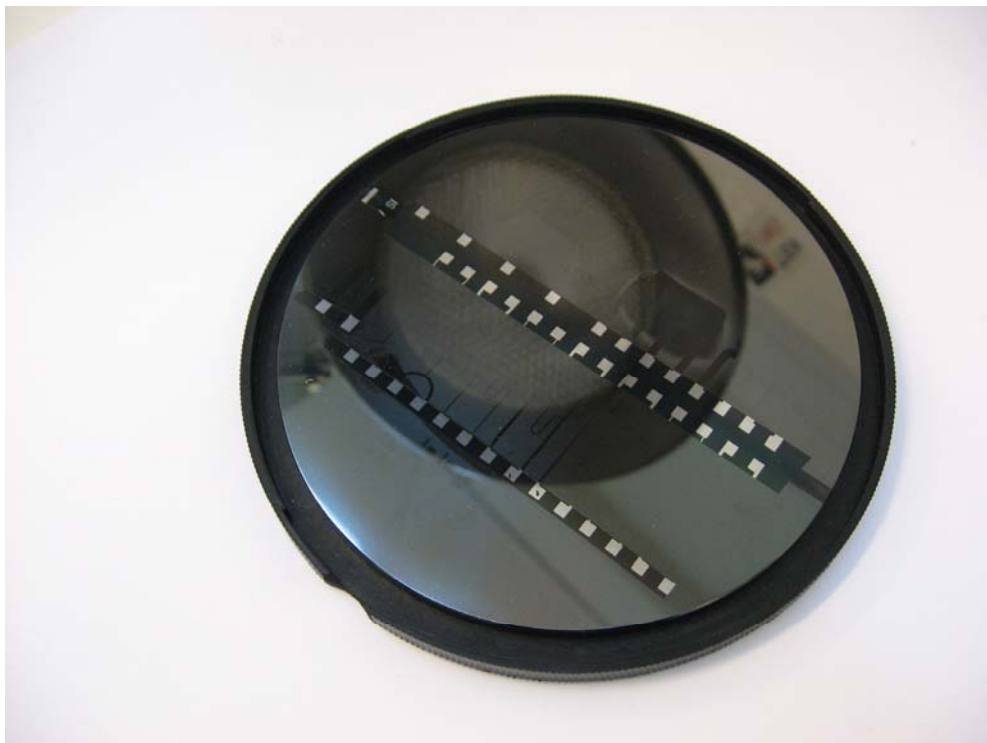
Figure 23: Buried “Pt100” temperature sensors under a low friction Diamond Like Carbon coating. Uncovered Pt bonding pads for electric connection can clearly be seen.
