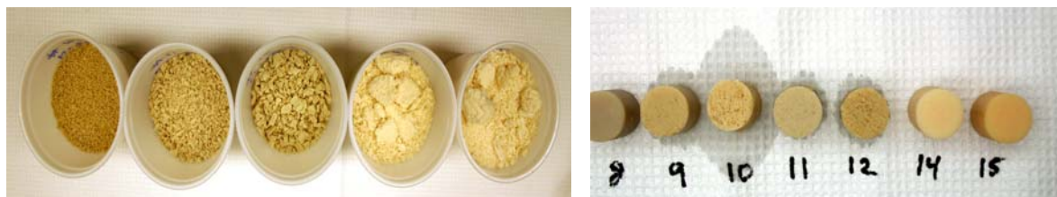
Figure 7.19. Left: Dried samples #10-15. Right: Gelled products of re-hydrated dried samples #8-15. Observe the wet area around sample 10.
