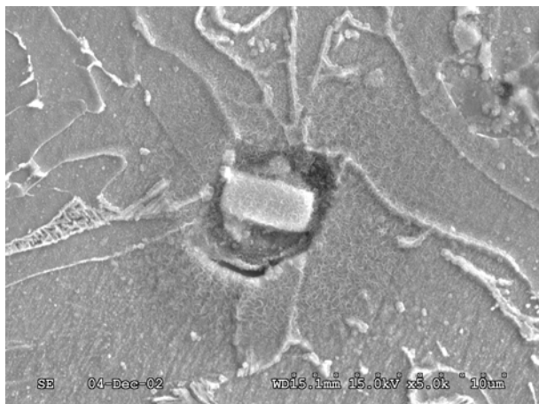
Figure 21. Inclusion in an etched sample of steel D4. The inclusion has nucleated acicular ferrite.
