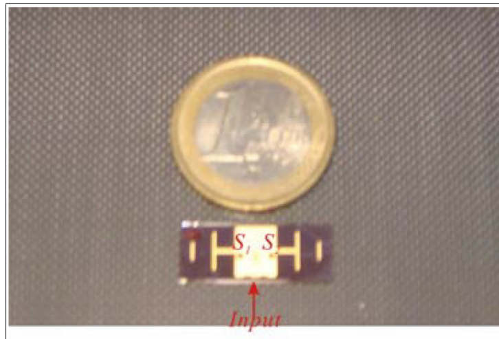
Fig. 13. Photographs of the array antenna integrated with RF MEMS based SPDT router on quartz substrate.
