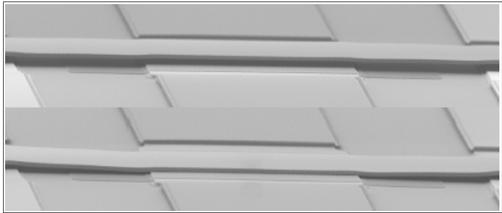
Fig. 6. SEM images of the fabricated main switch, in up and down state.
