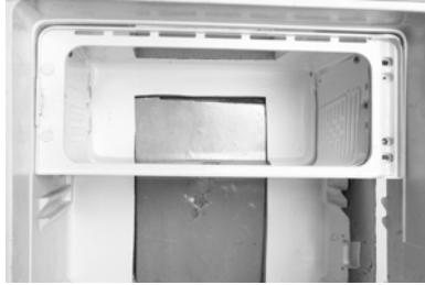
Figure 6 Inside detail of domestic refrigerator during manufacturing, showing the foam insulation.
