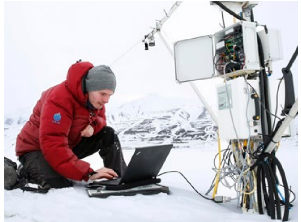
Norbert Pirk is a doctoral student at Lund University and the University Centre in Svalbard (UNIS). He uses flux chambers and other advanced technical equipment to study the production of methane and CO 2 in the tundra on Svalbard. Photo: NordForsk/Terje Heiestad
