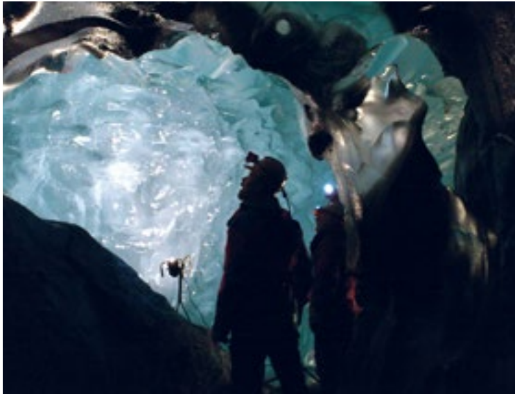
One of the access points to Svartisen Subglacial Laboratory allows the use of hot-water drilling to melt out ice tunnels in order to gain access to the glacier bed. Photo: Alexandra Messerli
