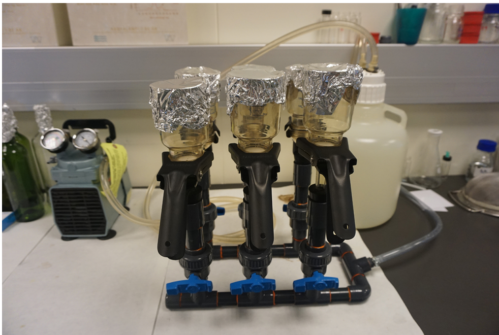
Figure 3: Filtration unit with an electricity driven vacuum pump (picture by Anne de Vries).
