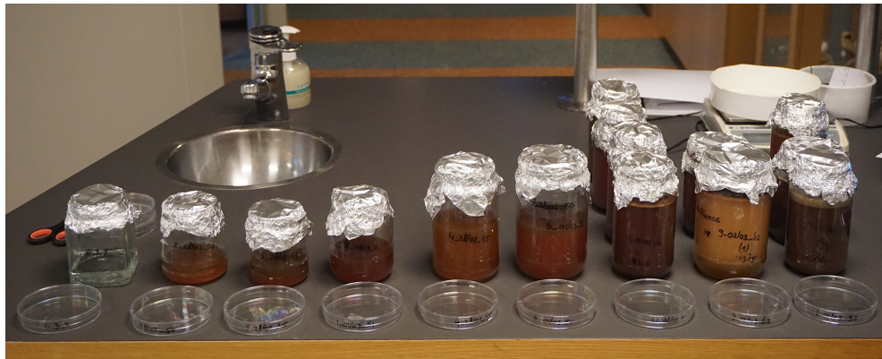
Figure 4: Jars containing dissolved fish guts covered with aluminium foil to prevent air contamination (picture by Anne de Vries).
