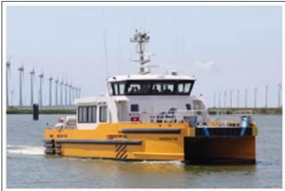
Figure 16 Crew transport vessel for carrying personnel to the SubFarm.
