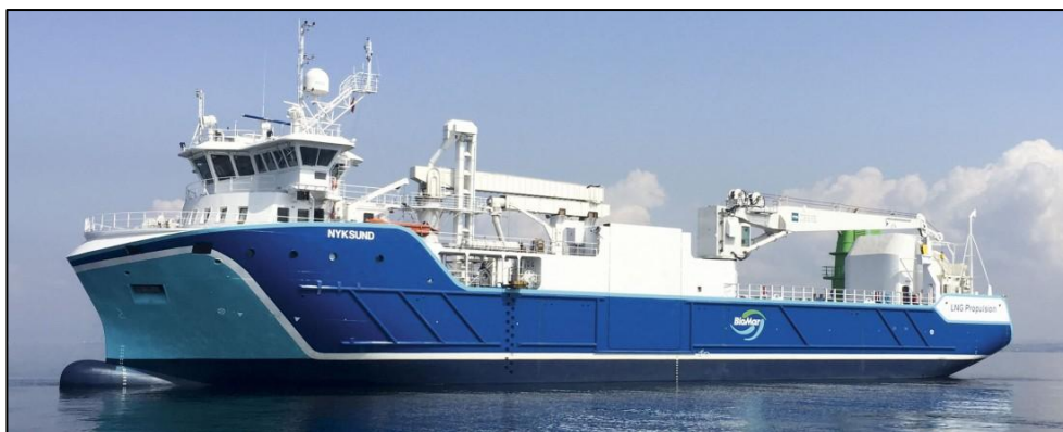
Figure 15 Typical pellets carrier for the aquaculture industry.
