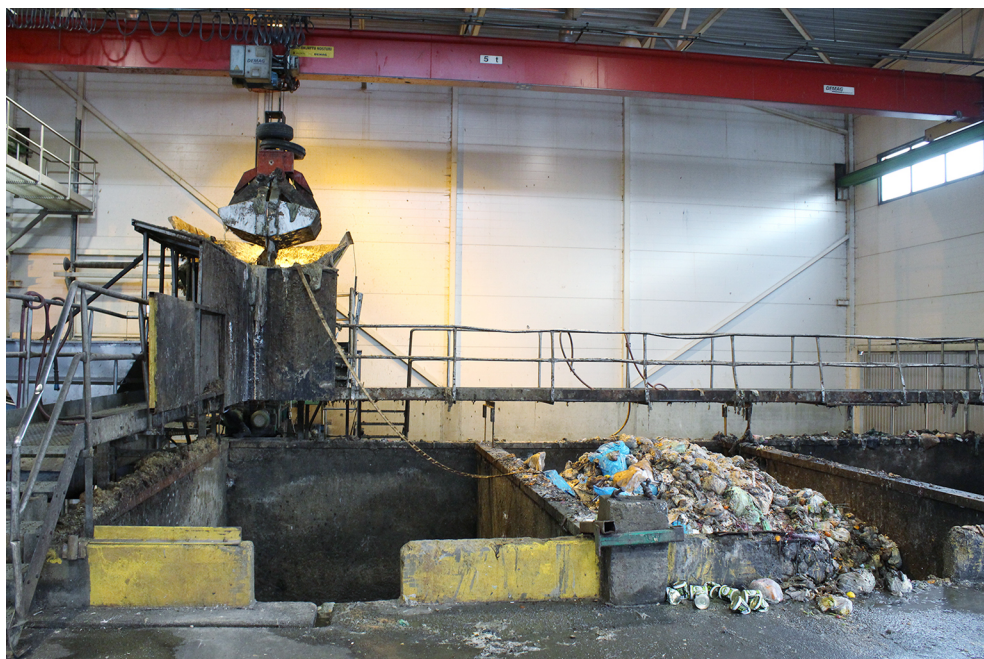
Figure 14: Indoor receipt. Packaging is removed before biogas treatment.
