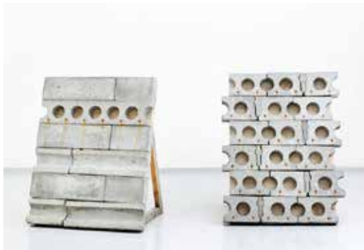
Figure 62 > Concrete bricks made from concrete slabs
