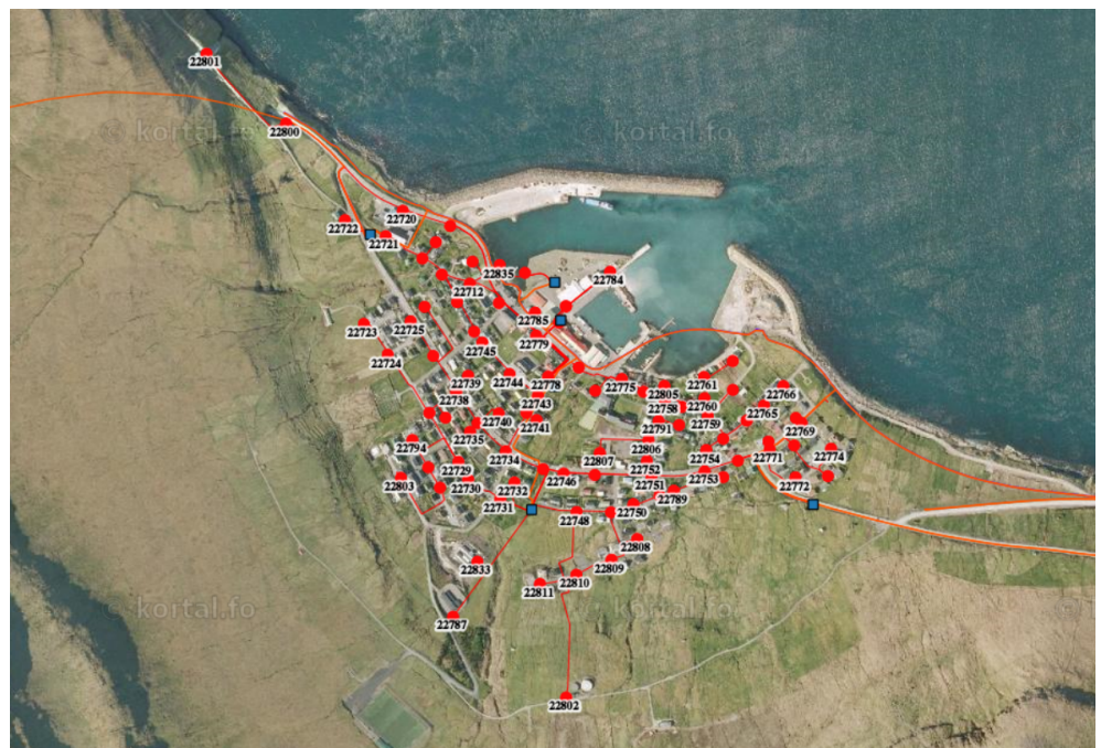
Figure 4.2 Electric grids in and through Leirvík. The orange line is 20 kV (from www.kortal.fo )
